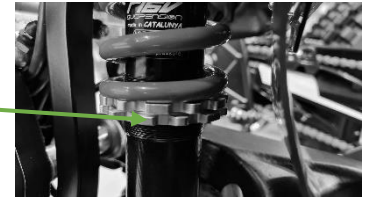
Figure 2 : Spring preload adjustment
